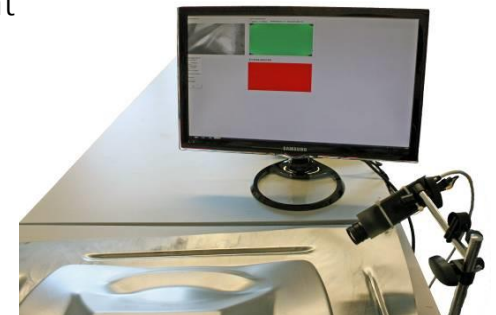
optical InLine control of finished parts
