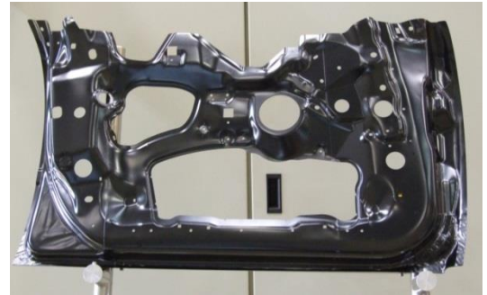
Inner door Magnesium Tailored Blank (AZ 31)
