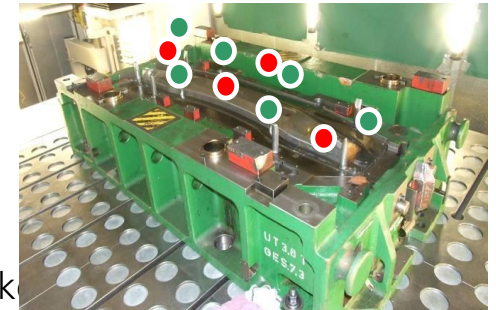
piezo sensors and sensors for structure-born noise
