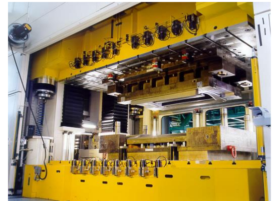
16 000 kN hydraulic Tryoutpress
